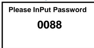
➤ Press MODE button, through UP and DOWN button , setup password 0088 , press SET button to save.
