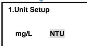
➤ Through UP and DOWN button, select unit, press SET button to save.
