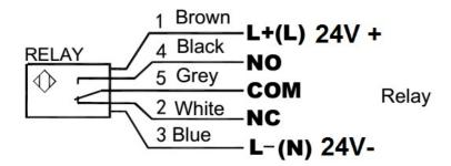
Power supply: DC24V, Switch signal: DC24V, 400mA max
